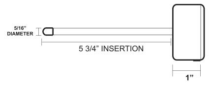
The "SAS" is constructed of UV stabilized Poly Carbonate Plastic with seamlessaluminum tubing frame and a highly accurate thermistor with 24AWG 12" leads. The unique construction provides a thermal barrier between the temperature probe and the duct work allowing precise air temperature measurements.
